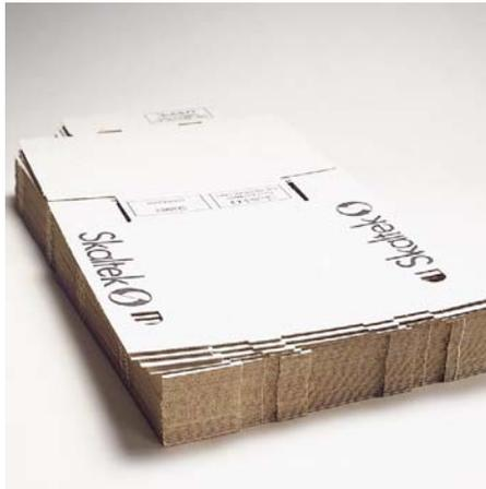
Coil Pac is made of cardboard. Pre-printed cardboard blanks are delivered from the supplier. A special Skaltek Carton Folder automatically folds the cartons, which are manufactured according to Skaltek's specifications.
